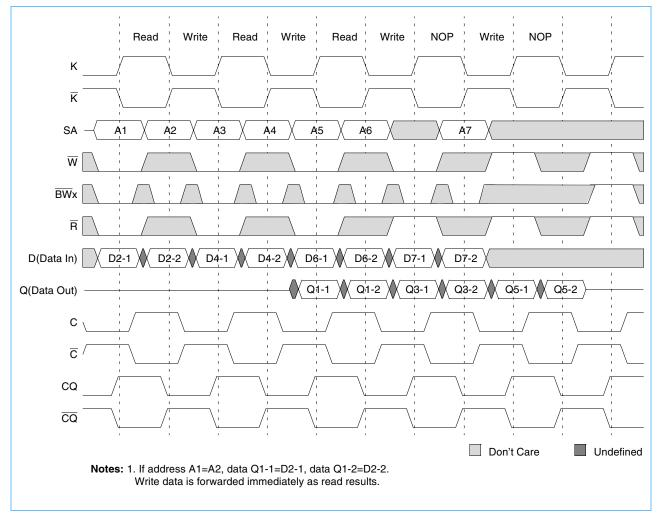
Read, Write, and NOP Timing Diagram
